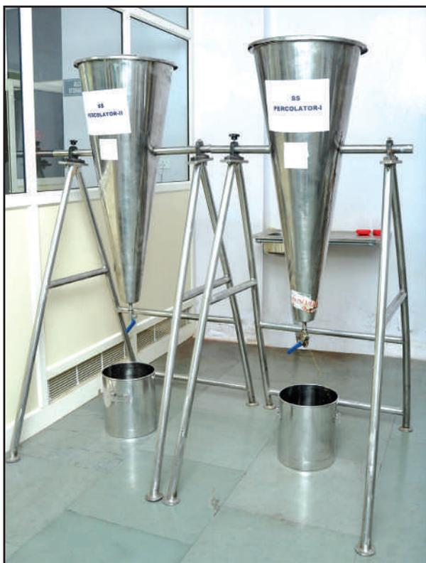
**Percolation-** It is a comparatively short process, but is a special method used for the extraction of dried vegetable and drug substances. This process is carried out in a special vessel known as the percolator. Mother tincture can be obtained directly. Decantation is not necessary before filtration.
